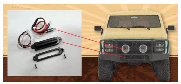
The LED light bar can be installed directly to the Rock Van bumper without use of the trim piece. The included supplemental trim piece allows use of the LED lightbar on other types and brands of bodies.
