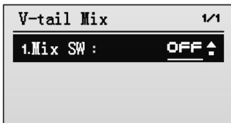
2. Modify the value of **Mix SW** to **ON** by pressing **R/+** key, to activate V-tail mixing function.
