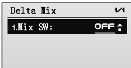
2. Modify the value of **Mix SW** to **ON** by pressing **R/+** key, to activate the delta mixing function.
