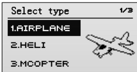
2. Press **UP** or **DOWN** key to select the model type, and then press **ENT** key to confirm the selection. The LCD display will back to **Model Set** interface automatically.
