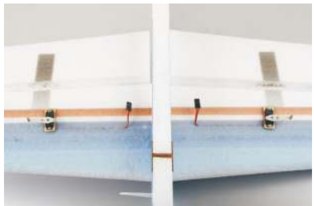
9. Use the same method to install the aileron servos.
