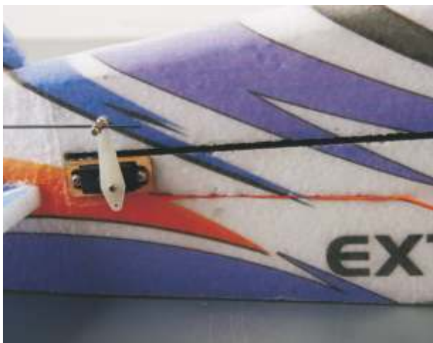
30. Embed the rudder and elevator servo leads into the pre-cut slots on two sides of fuselage. Pls use the servo extension wire if the servo wire is not long enough.
