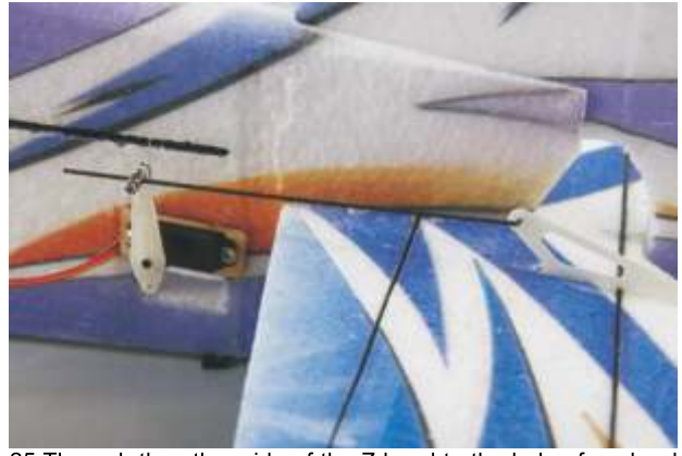
25. Through the other side of the Z bend to the hole of pushrod connector, and then insert the rudder and elevator horn into the pre-cut slot.
