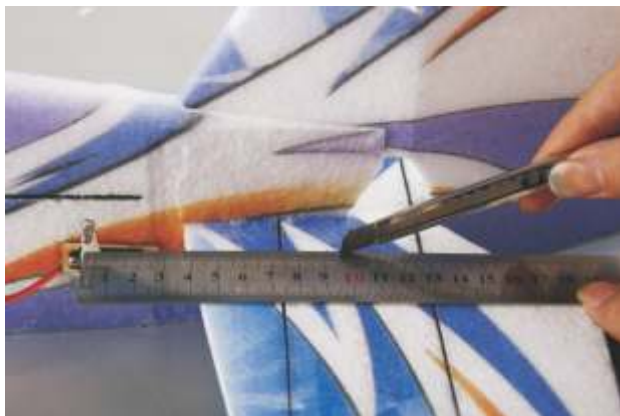
23. Use a hobby knife to cut a small slot on the elevator so that can install the control horn easily.
