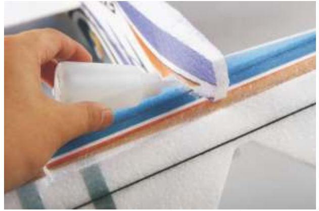
19. Drop some glue on the joints of elevator and fuselage to fix.
