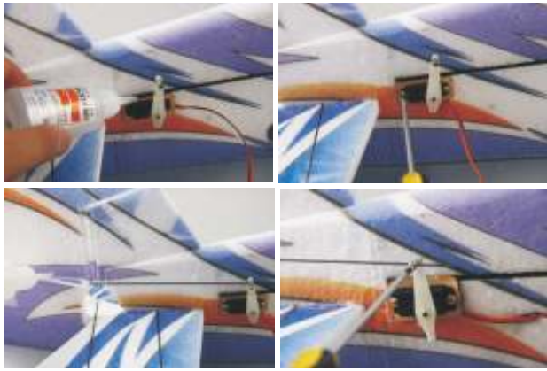
29. Use the same method of installing the elevator pushrod to install the rudder pushrod.
