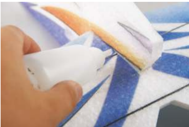
18. Insert elevator into the slot of fuselage. Make sure C=D (refer to the picture).
