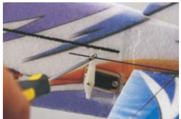
27. Use screwdriver to tighten the pushrod connector with the screws.
