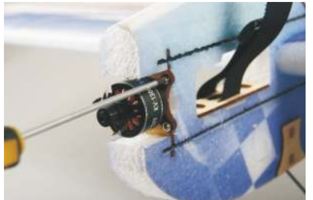
35. Use included screws to fix the motor onto the motor mount.
