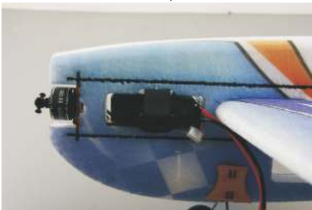
38. Insert battery into the battery hole.
