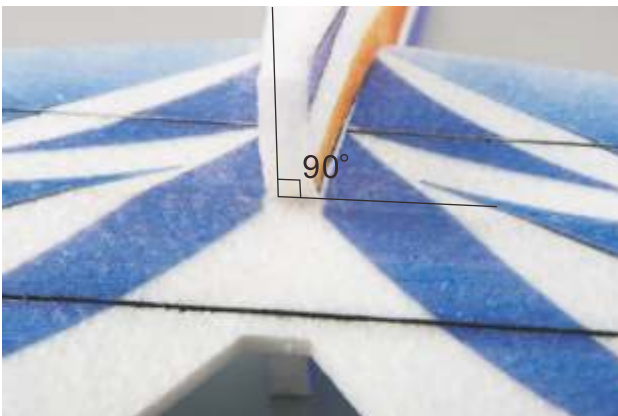
18. Insert elevator into the slot of fuselage. Make sure C=D (refer to the picture).
