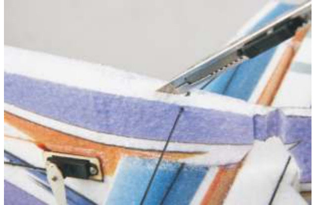
33. Use a knife to cut a slot under the fuselage .
