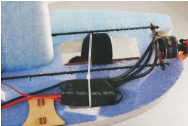
36. Connect motor and ESC, then adjust to correct motor running direction before flying. Put ESC into the slot of downside fuselage.
