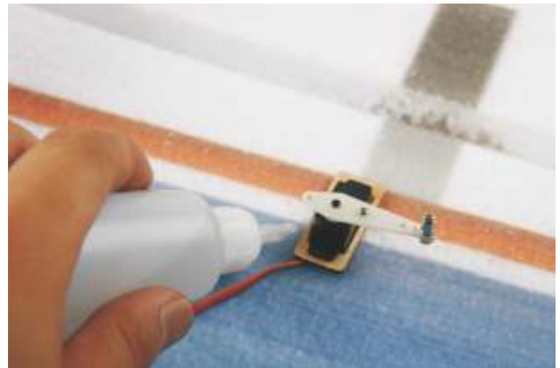
7. Put the servo into the pre-cut servo hole, then use glue to fix the servo mount onto the wing. Make sure the servo arm point to the wingtip.
