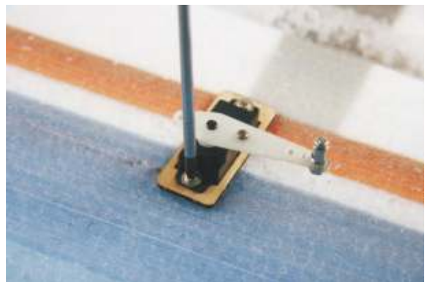
8. And fix the servos onto the plywood servo mount with included screws.
