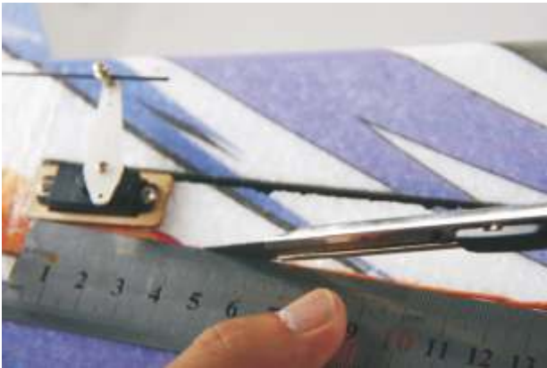
29. Use the same method of installing the elevator pushrod to install the rudder pushrod.
