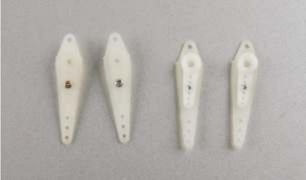
3. Fix the servo extension arm onto the servo arm with screw .
