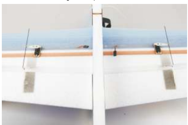
16. Use the same method to install the aileron pushrod.
