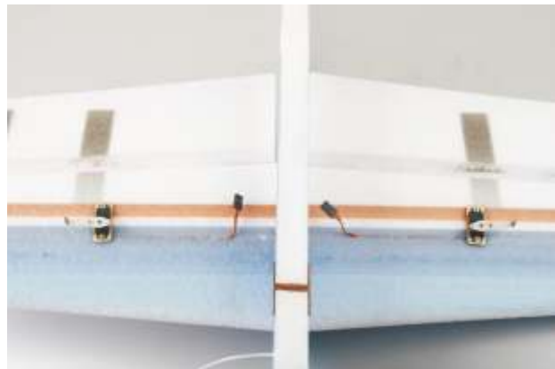
10. Use knife to cut slots on wing, then embed aileron servo leads as picture shown.
