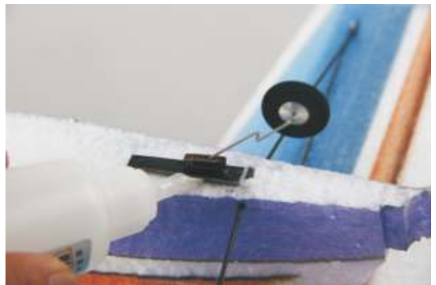
34. Glue the tail wheel set into the fuselage slot .
