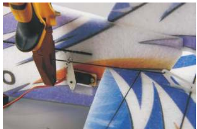
28. Use the pliers to cut off the superfluous steel wire.
