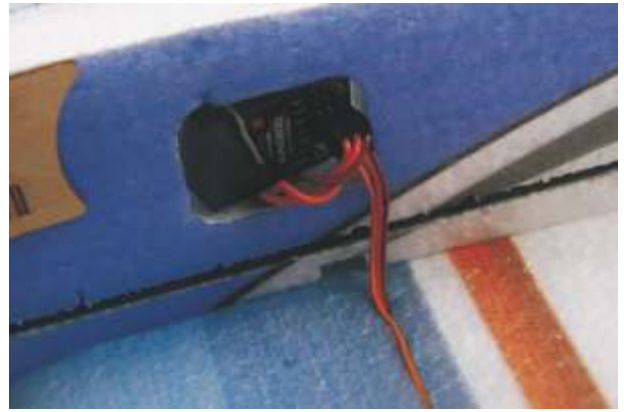
40. After test, put the receiver into the receiver slot. (see picture)
