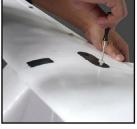
4 Fix the wing on fuselage
