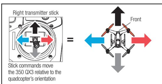
Stick commands move the 350 QX3 relative to the quadcopter's orientation
