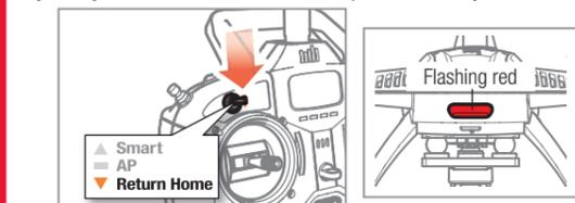
The 350 QX3 will return to the start position, land and stop the motors. You may cancel the return to home function by switching back to Smart or AP Mode on the top left switch on your transmitter.
