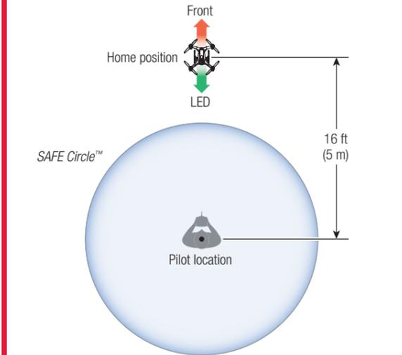
**CAUTION:** When the home location is set, the 350 QX3 must be approximately 16 feet (5 meters) from where the pilot will stand during flight, pointing away from the pilot. If the aircraft is pointed in any other direction, the SAFE Circle feature will not function as expected and may result in personal injury or damage to property. Once the aircraft's motors are started, do not change your position.
