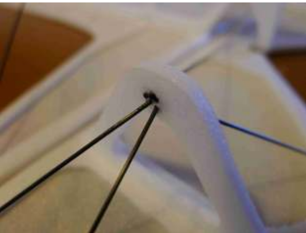
Fix with C/A the 0,8 mm carbon rods to reinforce the elevator.
