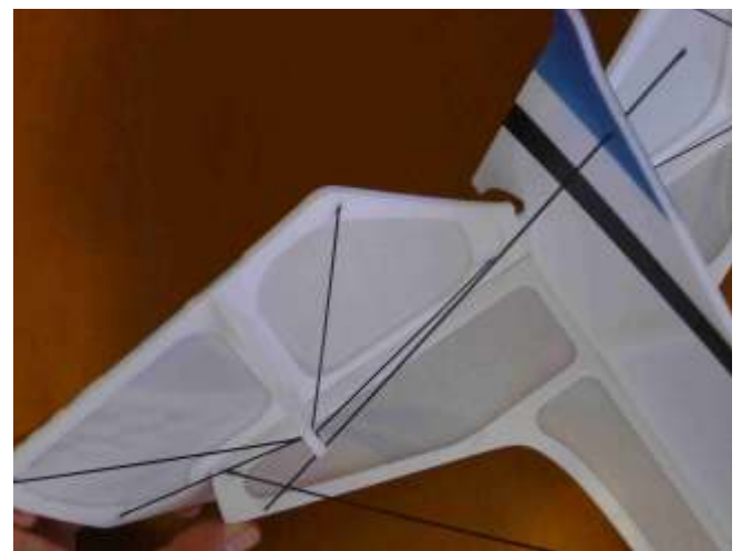
Fix with C/A the 0,8 mm carbon rods to reinforce the ailerons.
