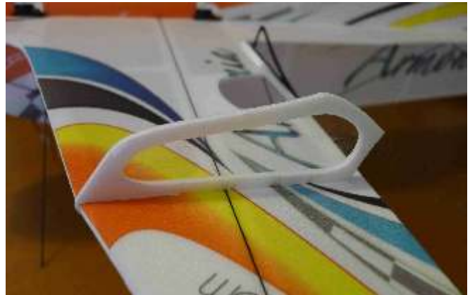
Insert the upside vertical winglets into the pre-reserved slots on the upside of the wing and apply some C/A to fix.
