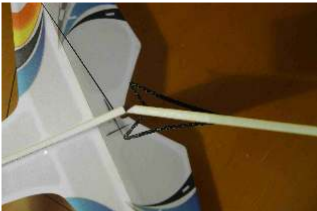
Insert the 0,5 mm x 4 cm carbon strip in the elevator control horn. Then glue them together in the pre-reserved slot. ATTENTION: elevator and rudder control horns are asymmetric. The shorter part goes on the side of mobile surface where there is the 50° bevel for movement.
