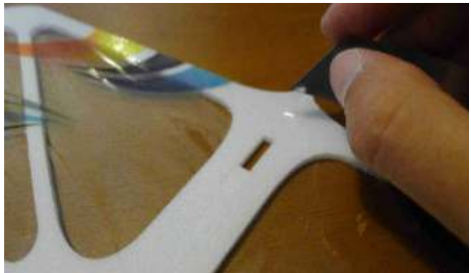
Insert the upside vertical winglets into the pre-reserved slots on the upside of the wing and apply some C/A to fix.
