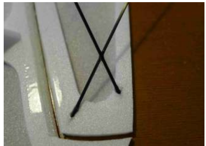
Install the 1 mm x 18,5 cm carbon rod paying attention to the elevator deflection. ATTENTION: elevator, when moves down, must not touch this carbon rod!
