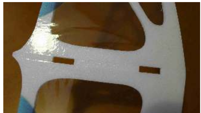
Remove with a cutter 3 mm of transparent film from the bottom horizontal winglet.
