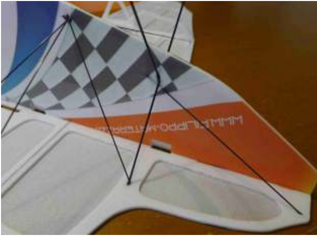
Fix with C/A the three 1 mm carbon rods as shown in the picture.
