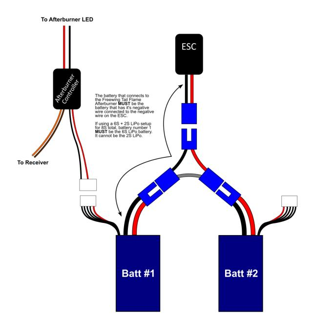
2. Note which battery has its ground (black) wire connected directly to the ESC's black wire and use the balance tab from this battery to connect to the Tail Flame Afterburner. Connecting the other battery's balance tab to the afterburner will cause the system to fail, and potentially cause a fire. If using a 6S and 2S battery in series for 8S, be sure to connect your 6S battery's negative (black) wire to the ESC's negative (black) wire.
