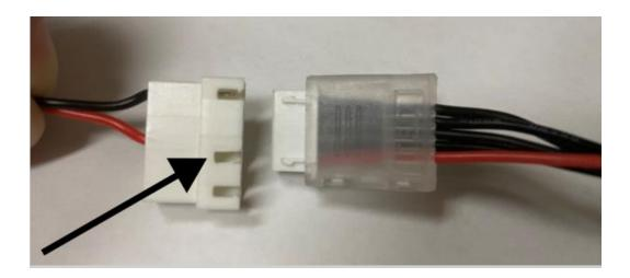
• If using two 4S LiPos, you can cut a small notch in the connector of the Tail Flame Afterburner to allow the 4S balance tab to connect more easily.
