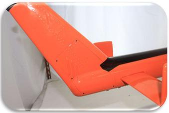
Then screw the tail fuselage onto the front fuselage.
