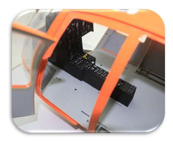
Next, install the cockpit levers (44, 45, 46) according to the cutouts on the floorboard, securing them with epoxide
