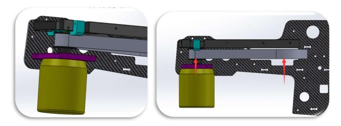
Now tension the belt with the turquoise block by tightening the two front facing screws. Attach the other side frame, and adjust the motor main shaft until it is perpendicular to the belt. Then tighten all four screws of the violet motor holder. Then tighten the 4 screws that hold the top motor shaft bearing block.
