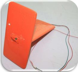
Next, thread the cables into the tail and then glue the tail units in place. Ensure they are mounted perpendicular onto the tail boom.
