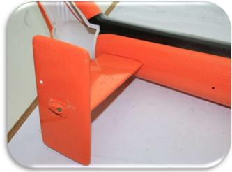
Use glue to fix the wires in place as shown. Next adjust the fins so they are correctly angled to each other and perpendicular to the tail fin. It's important to take care with this step, as a poorly adjusted model will look unattractive. When satisfied with the placement, apply sufficient glue to both insets and attach the stabilizers securely to the boom. Ensure a strong bond is achieved.
