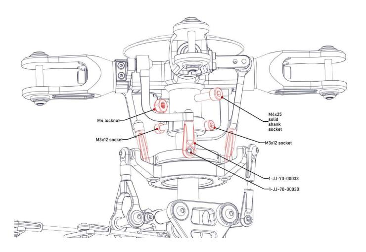
Ensure that the distance between the ball link and the L lever is 24mm on all sides. Finally, attach the ball links (70-00025) onto the swashplate's upper disc uni-links (70-00030) by snapping them in place.
