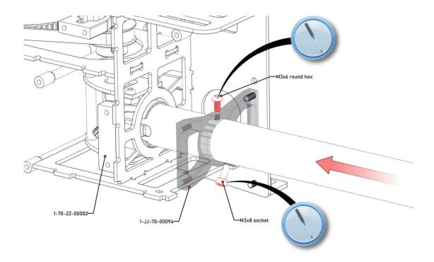
Finally, attach the carbon support beams onto the main frame and the tail boom clamp according to the provided illustration.
