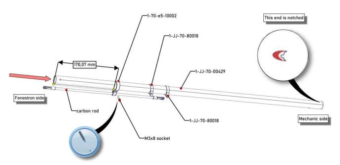
Then, insert the tail boom into the tail boom holders (1-70-ZZ-00002, 1-JJ-70-00094). Secure the tube in place with screw M3x8 via the clamp up and additionally with screw M3x6 as shown. Finally, attach the carbon support beams (70-00104-70-00106) onto the main frame and the tail boom clamp (600UH1-007).
