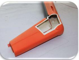
Connect the red LED (53) with the 90mm extension cable (54) and mount the LED in the fuselage with glue. Glue the cap (55) on.
