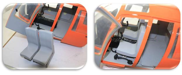
Next, proceed to install the back seats (50) according to the cutouts on the floorboard, securing them with epoxide glue.
