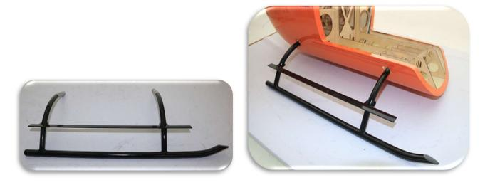
Next, utilize the four screws (35) and washers (27) to fasten and secure the landing gear in place, on both sides in the back and in the front locations. Please exercise caution and avoid overtightening the screws.
