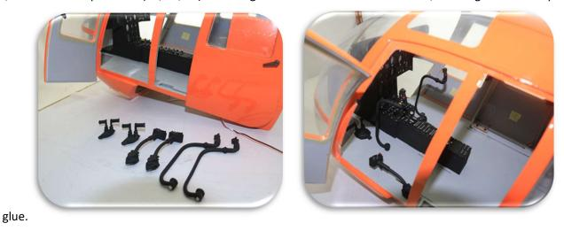
Next, proceed to install the front seats (49) according to the cutouts on the floorboard, securing them with epoxide
