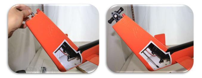
Then connect the linkages on the tail gearbox so that the servo controls the tail rotor pitch again. Close the tail hatch with the screws.
