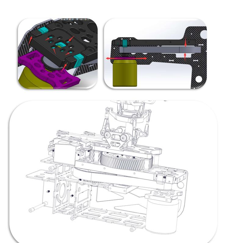
Use both tensioning screws to adjust the belt drive tension. The belt should not be too tight to avoid unnecessary wear. After installing the motor, reassemble the side frames.
