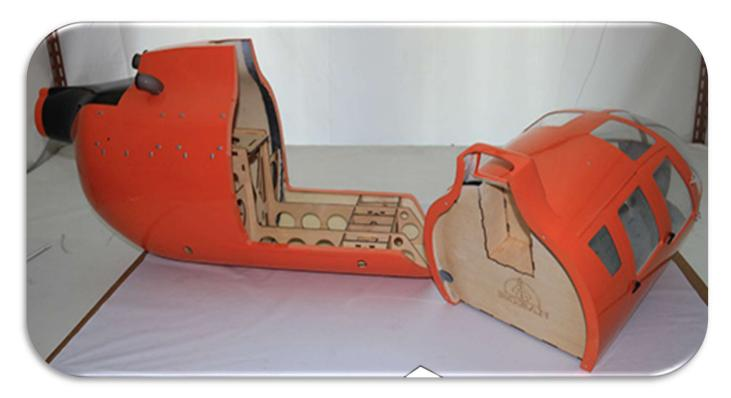
The front section is secured by magnets and two screws, which hold it in place.
