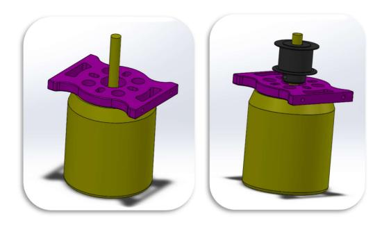
Now insert the pulley into the belt and install the mount onto one side of the main frame, but do not tighten the screws yet. First, make sure that the height of the belt is adjusted correctly. If the belt runs too low, it will damage the 2<sup>nd</sup> stage gear for the tail drive. When aligned, tighten the pulley set screws.
