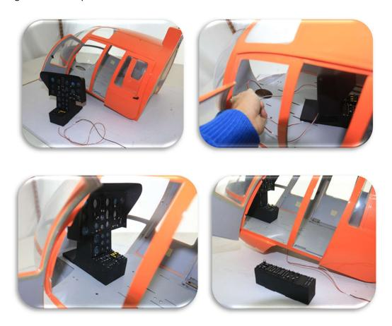
Then glue the center console (48) onto floorboard as shown.
