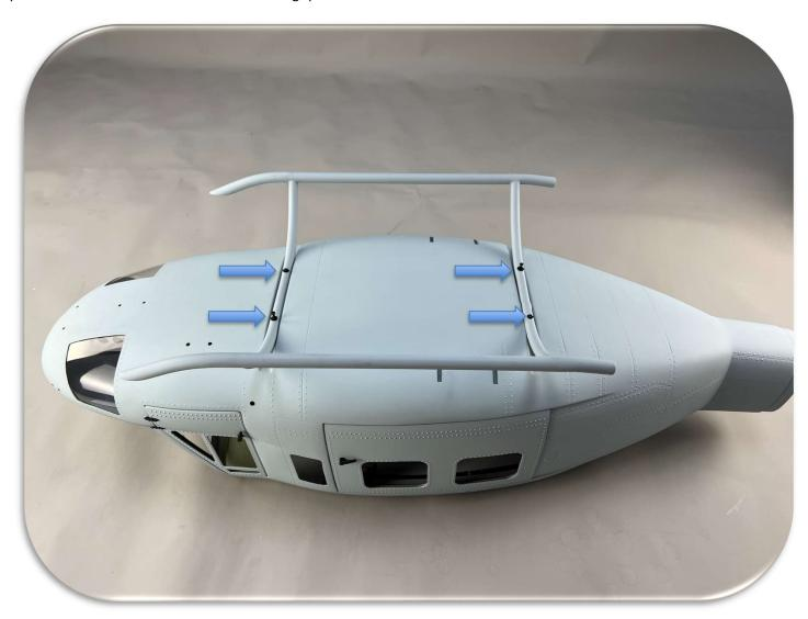
Next, utilize the four screws (38) to fasten and secure the landing gear in place. Please exercise caution and avoid overtightening the screws.
