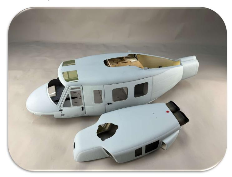
The top section is secured by magnets and two screws, which hold it in place.
