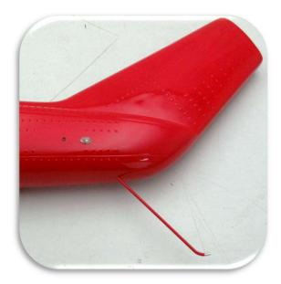
Next, install the LED (58) in the top cover as shown with glue. When the glue settled, attach the cap (60) with glue as well. Secure the wire on the side downwards to where you intend to install the light controller with small dabs of hot melt glue.
