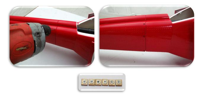
Open the tail access hatch and insert the short shaft into the angled gearbox first. Then insert the short boom with the tail rotor attached to it as shown. Tighten the screws on the gearbox that hold the short boom in place after making sure the tail rotor is perpendicular to the front mechanics.
