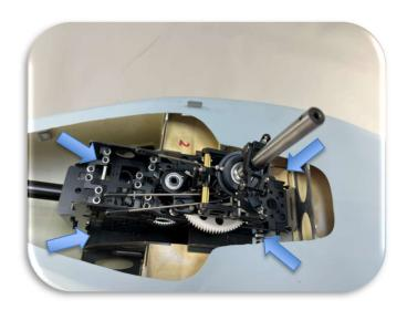
Then screw the tail fuselage onto the front fuselage. Make sure to connect all LED wires with the controller, and that all electrical components are connected. Finally, make sure that the battery cable reach the battery compartment. Only then install the engine hatch and secure it with screws. Finally mount the main rotor head onto the main shaft.
