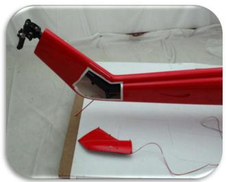
Use the screws (M3x16 socket) and washers (M3) as shown to secure the mechanics in place.
