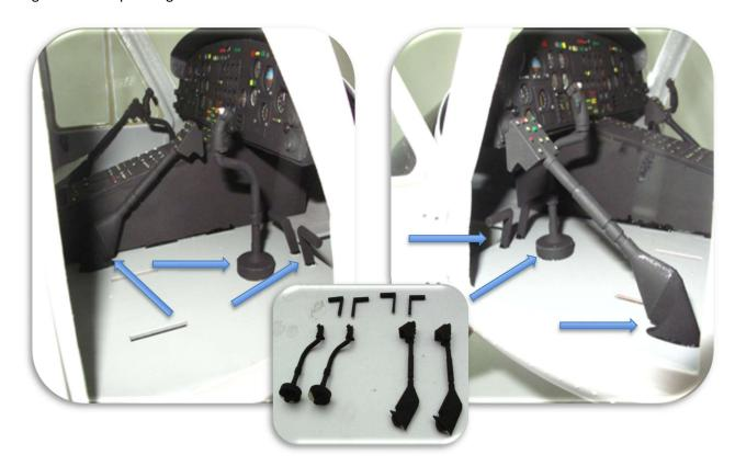
Next, proceed to install the front seats (67). First glue the backside plywood frame onto the seats. After the glue settled secure the seats, according to the cutouts on the floorboard, with epoxide glue.
