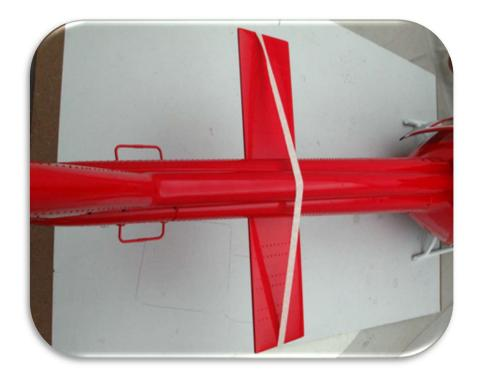
Now your mechanics should be properly set up inside the fuselage. Make sure that when rotating the tail and main rotor there is enough clearance for all moving parts to the fuselage.
