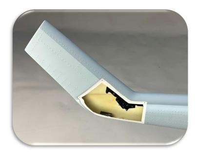
Next, secure the socket of the white LEDs (55) with a small amount of transparent epoxy or acrylic glue on both the hatch and the tail boom. Once the socket's glue has settled, secure the cap (39) of the LED with glue as well. Then connect each of them with a 90mm extension cable (54).
