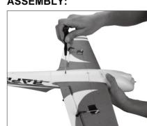
Install the wing with PM3\*25mm screw.
