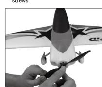
6 Install the propeller.
