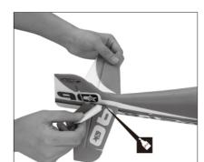
Apply some glue on the contact area on the elevator. Glue the elevator onto the fuselage.
