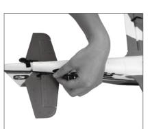
Install the elevator push rod as shown
