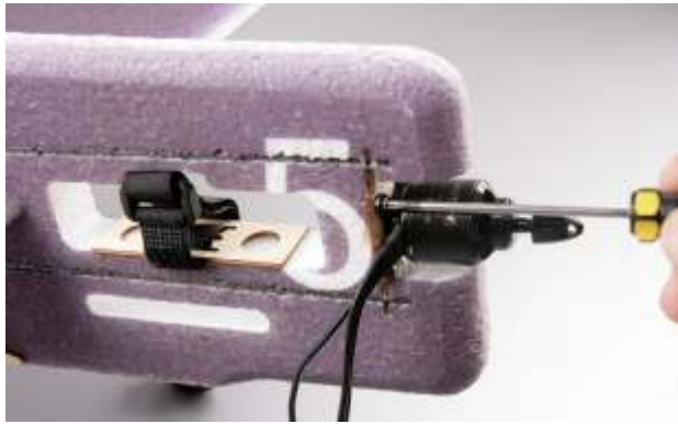
29. Use included screws to fix the motor onto the motor mount.
