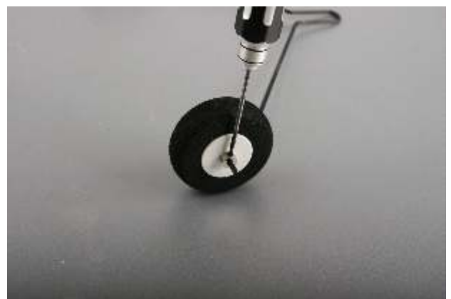
27. Install wheel blocks to fix wheels.
