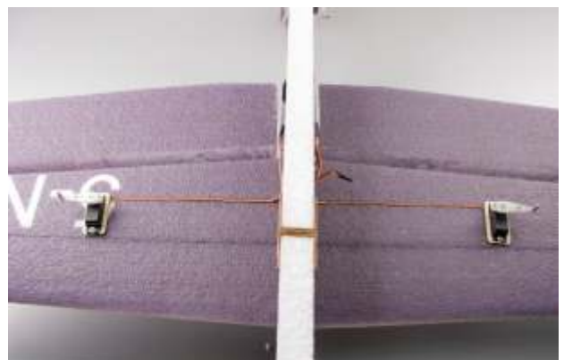
12. And fix the servos onto the plywood servo mount with included screws. Use knife to cut slots on wing, then embed aileron servo leads as picture shown.
