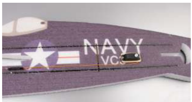
6. Embed servo leads into the slot.
