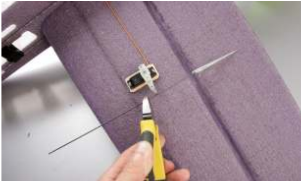
24. Reserve proper length of Z bend, then cut off additional part that you don't need.
