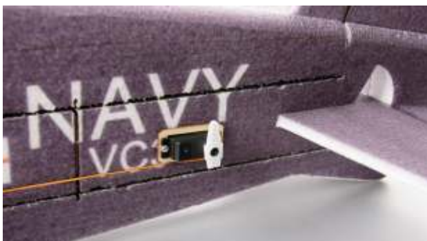
18. Same operation on elevator & rudder servos.
