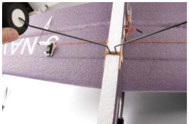
28. Insert landing gear frame into the slot on bottom fuselage, please refer to picture.
