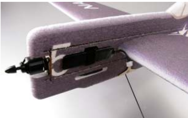
31. Insert battery into the battery hole.
