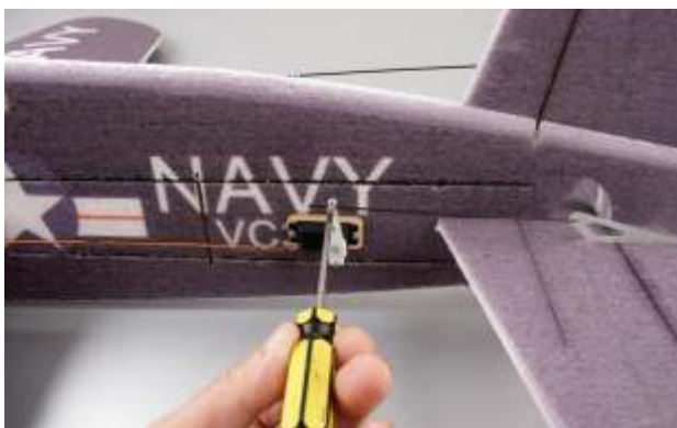
25. Put one end of steel wire into the hole of adjustor, then fix with screwdriver.
