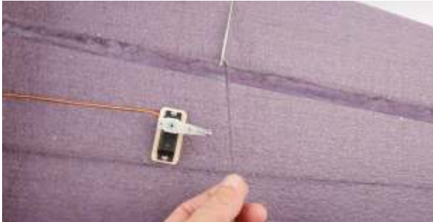
23. Connect Z bend into the hole of control horn.
