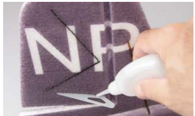
22. Cut a slot on control surface along a ruler, and insert control horn into this slot, then use CA to fix. The same operation on aileron, elevator & rudder control horns.
