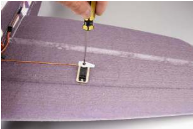
17. Fix trimmed servo arm with included screw.
