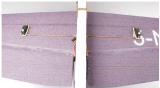
20. Fix servo arm extension on servo arm with 2pcs 2*4mm self tapping screws.
