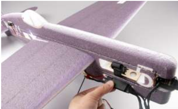
30. Connect motor and ESC, then adjust to correct motor running direction before flying. Put ESC into the slot of downside fuselage.
