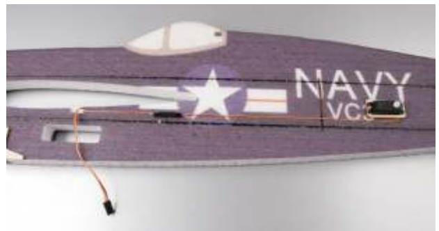
5. Cut a 10mm length slot on fuselage along a ruler, and make sure servo wire can be embedded deeply into the foam.
