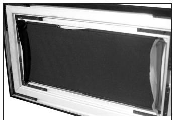
4. First install the two long sides, then the short sides to provide a perfectly tensioned surface.
