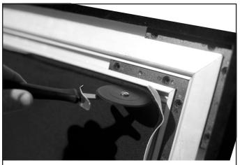
3. Use a regular pizza-slicer to insert and fit the fabric into the attachment profiles.
