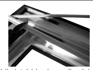
1. Cut the included attachment profiles to fit the four sections of the frame.
