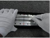
First, attach the long sections and secure them by tightening the screws
