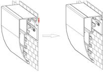
Then you simply hang the frame onto the two brackets and slide it into perfect position.
