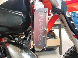
Once both sides are installed, secure the spark plug wire and the radiator overflow hose in their stock locations.
