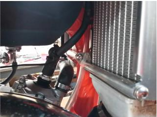
Take a moment and double check your work. Make sure all bolts and hose clamps are tight and no wires are pinched.
