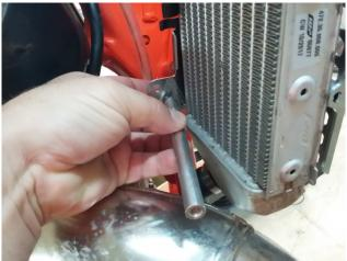
Slide the entire guard/radiator assembly on the frame and connect the upper radiator hose. Secure the radiator to the frame using the stock mounting bolts and the large nylon washers included in the hardware kit. Tighten the coolant hose clamp.
