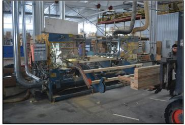
Roof Rafter Cutting Machinie Ensures Accurate Cuts Every Time
