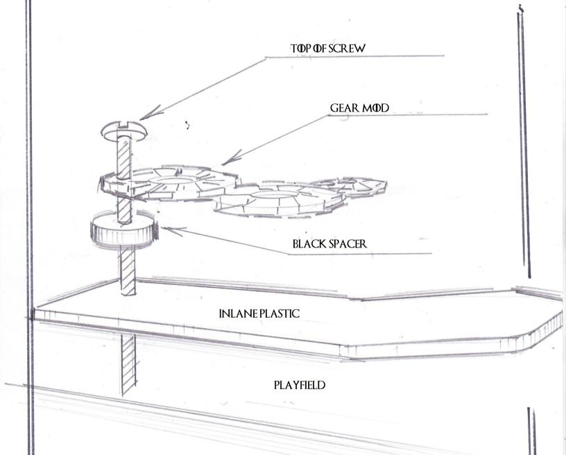
Remove the glass and lockbar, place a small towel on the playfield to protect it while working on your game. Use a phillips screwdriver and remove the inlane screws. Put the long screw through the gear mod hole then place the black spacer on the other side. Put these pieces back down and tighten screw down as indicated in the diagram. Do NOT overtighten. A snug fit will usually do it. If gears slip, just retighten when necessary.
