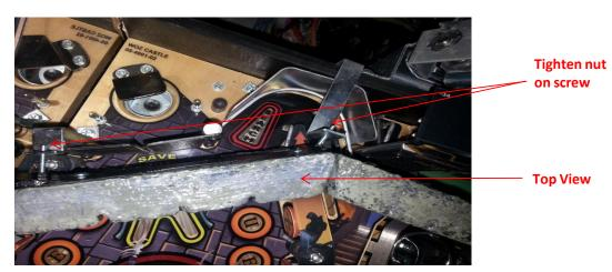
4 Install angled bracket (provided) by removing the existing nut # 3
