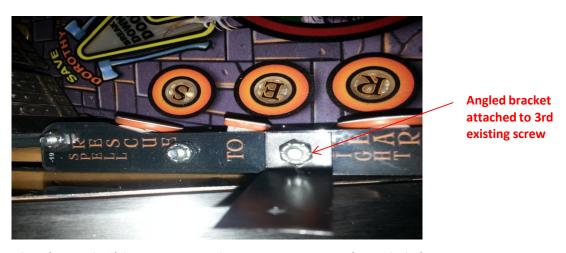
5 Install L bracket (provided) by removing the existing nut # 5 (spot light)
