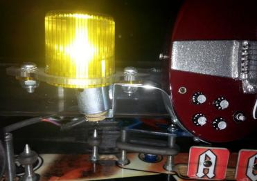
7. If your mod is game interactive, remove the balls, lift the playfield, hook up the alligator clips at the end of the enclosed LED strip to a near by flasher, pull the strip through any desired target opening and attach it to the back of the guitar with the provided 3M tape.
