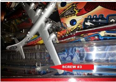
3. Take some screws off the plastic in order to loosen it just enough to be able to get needlenose pliers under it
