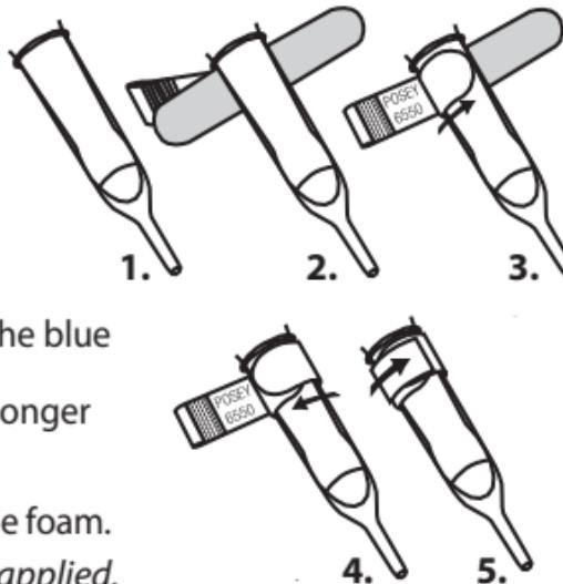
**A WARNING** DO NOT pull elastic too tight. Foam should not be compressed when applied.
