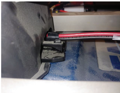
Figure 8 – Push the connector into the cavity
