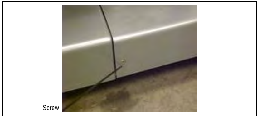
Figure 5-9. Install Base Cover Insert and Attach to Base Cover
