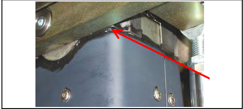
Figure 5-7. Seal Around Upper Plastic Covers and Column
