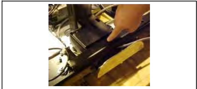
Figure 5-2. Apply Tape to Mounting Bracket
