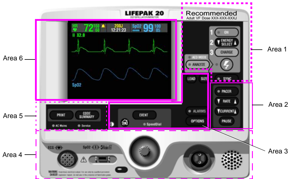
Figure 2-2 Front View without Door
