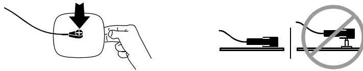
Figure 5-4 Connecting FAST-PATCH Electrodes to Defibrillation Cable
