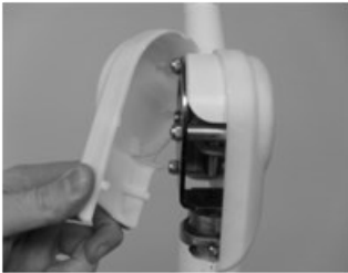
Step 5: Pry the LH cover forward.
