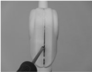
Step 3: Turn driver 90° to separate the covers.
