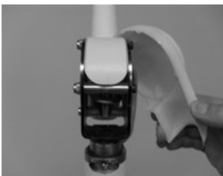
Step 7: Pry the RH cover forward.
