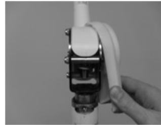
Step 6: Pry the RH cover up.
