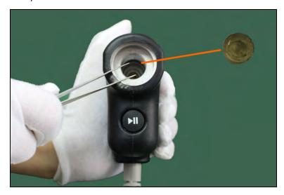
Step 3: Put a new spacer into the handpiece and make some adjustment with a tweezers. Make sure the spacer is
