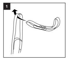
Take the sling extension strap and thread part way through the top loop of the sling strap ensuring correct attachment to both hoist and sling (see label).
