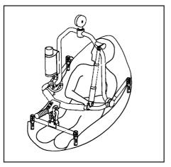
Move the 4-point cradle into position above the patient. Attach the amputee spreader bar. Keep the 4-point cradle away from the patient's face. Attach the shoulder strap and leg loops to the respective front and rear hooks on the 4-point cradle and the amputee spreader bar.
