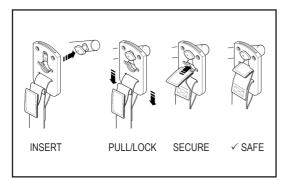
This sling is connected to the 4-point cradle and amputee spreader bar (shown right) using the Securi3 clip system which prevents inadvertent detachment. Follow the steps above to attach the sling. To remove, simply reverse this procedure.
