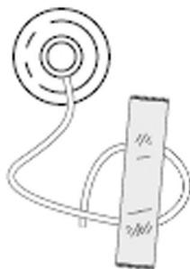
A secured stress loop prevents leadwire rotation about the electrode snap, leadwire tugging at the electrode, and ECG artifact.
