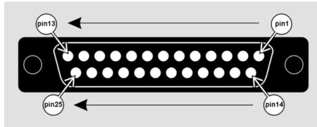
*Pin-out of the Electrocap connector for the S7000 Bedside Unit*
