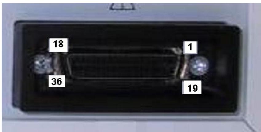
*Pin placement of the Unit Interface*
