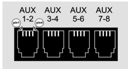
*Pin placement of the auxiliary inputs*
