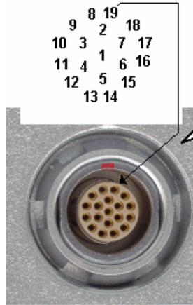
*Pin-out of the Communication Unit Interface (Fischer connector)*
