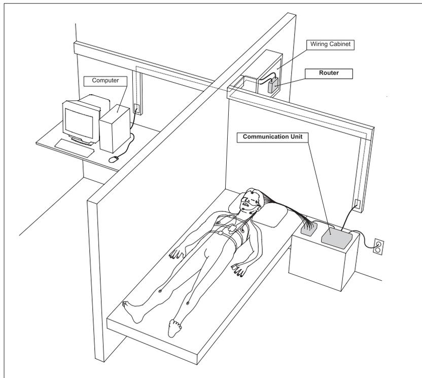
Most routers have a small green LED close to each port, which lights up if a device is connected to that port. After connecting all the devices and turning them on, make sure that the corresponding LED lights up on the router. In case the acquisition computer needs to be connected to a larger network, a second Ethernet adapter may be added to the computer.
