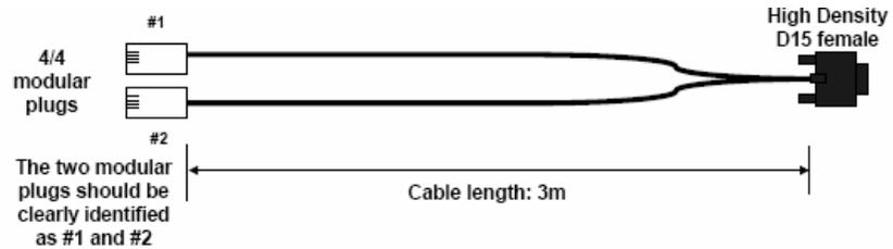
*Schematic of the Embla to TCM4 CO<sub>2</sub> Monitor Cable*
