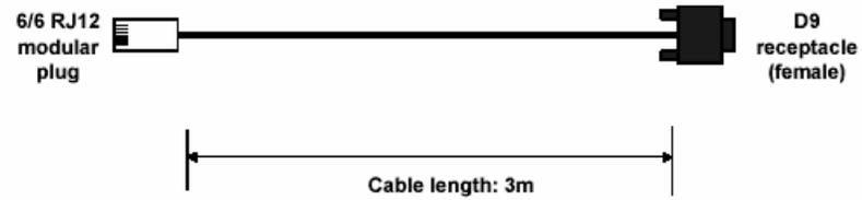
*Schematic of the Embla Serial Cable*
