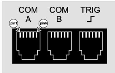
*Pin placement of the COM and Trigger ports*
