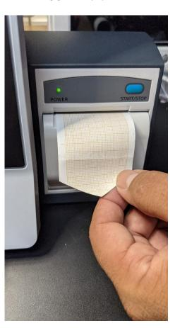
6. Turn module on in user maintenance area- enter user password (ABC standard or custom user password) ->module select ->recorder on (u)
