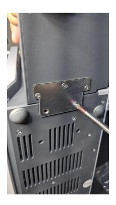
4. Place white section of printer back inside frame, and screw back into place
