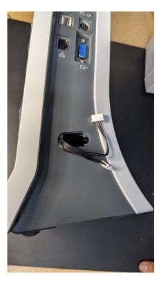
2. Take out two screws on inside of printer door, take out roller and white section of printer. Take wire from unit and thread through the side of the printer.
