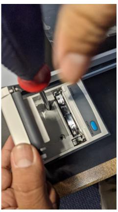
5. Insert paper- open door, have some paper lie on top of roller (DO NOT THREAD THROUGH ROLLER) and close door. Red grid should be showing/facing up if you are using gridded paper.
