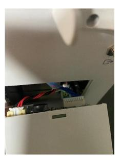
2.Slide printer into slot and screw into place.
