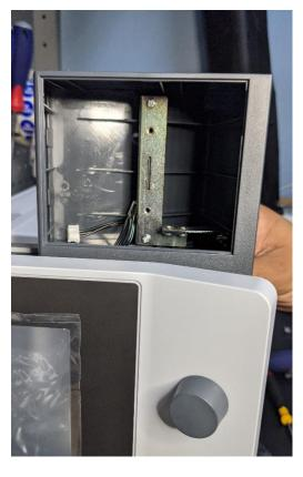
3. Secure printer onto bottom of unit
