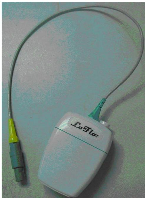
Figure 9-1 LoFlo CO<sub>2</sub> Module
