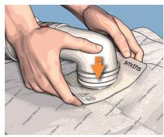
Attach the hose, ensuring the hose ridge snaps into the blanket collar ring.
