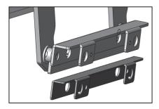
5. Re-insert the metal pins from the outside edge of the bed through the mounting holes and secure with snap rings on the inside edge of the bed. Make sure the snap rings are positioned in the groove of the metal pins.
