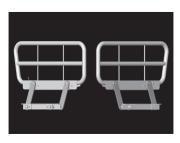
Unclip and remove the metal pins from the rail mounting brackets. Hook the rail bracket onto the edge of the bed decking. Align the rail bracket mounting holes with the bed decking mounting holes.
