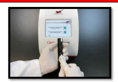
2. Clean the strip bed with a 70% alcohol solution. Avoid wiping the white color block on the top right side of the strip bed and avoid cleaning the groves on the left side of the strip bed. Dry the strip bed completely with a lint free tissue or clean cotton swab.
