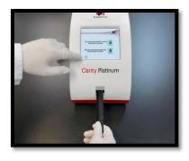
**3.** Return the strip bed into the device by seating it back into the groove until you feel pressure and it stays in the machine by itself. Press the bottom arrow  $\bigcirc$  on the screen and the strip bed will be retracted.
