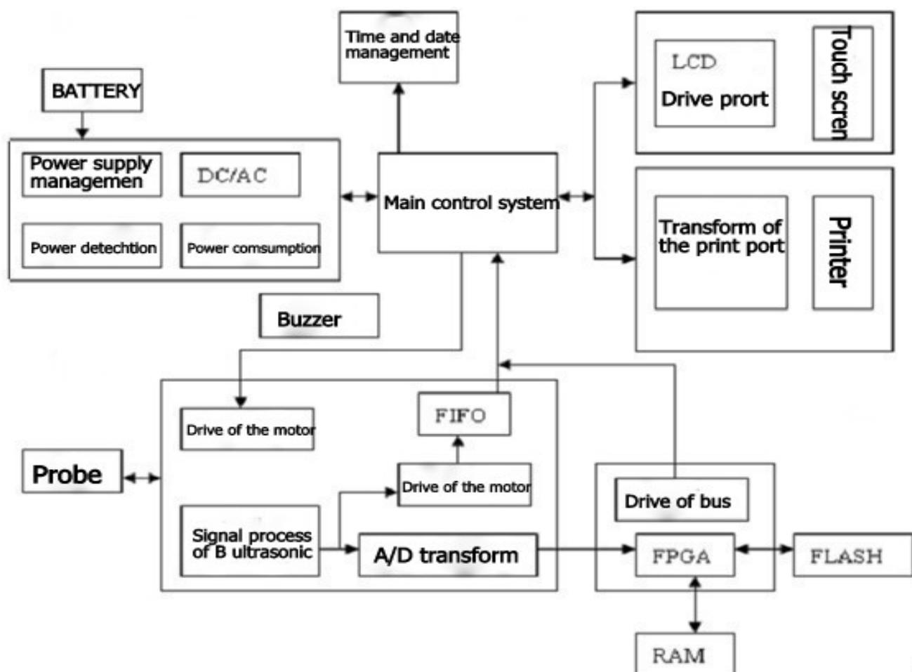
Figure 3-4 PadScan HD3 electricity principle diagram
