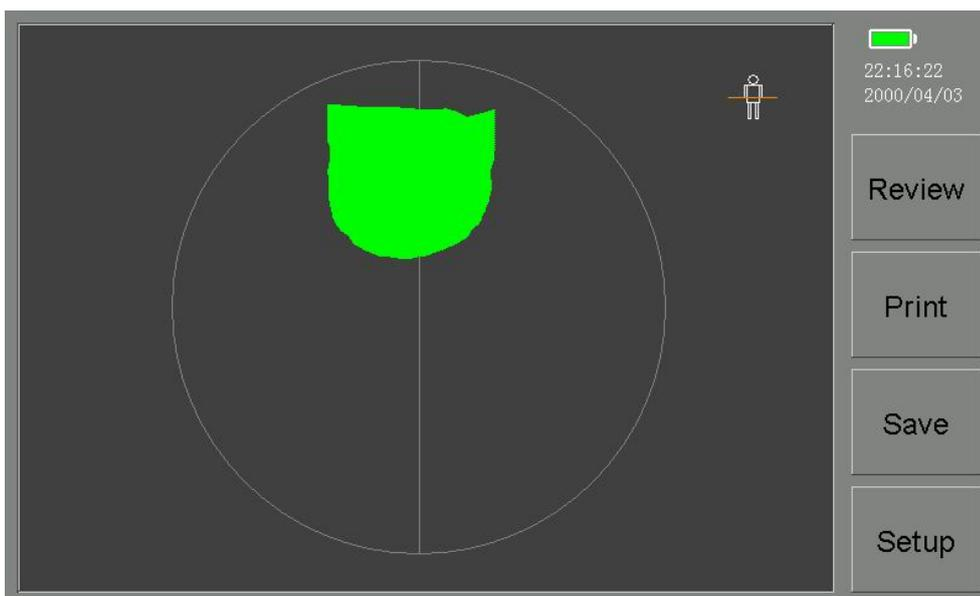
Figure 5-2-2 PadScan HD3 Easy Mode bladder scanning interface
