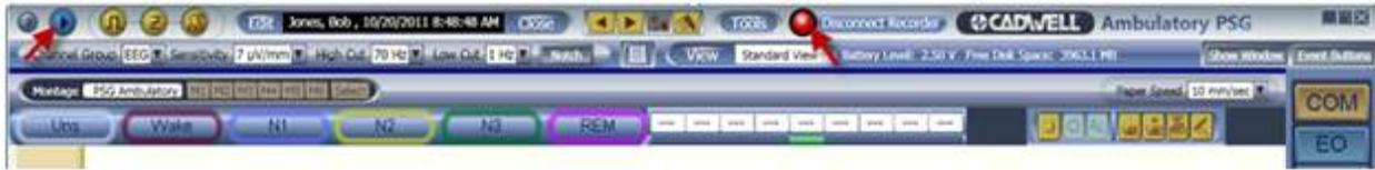
2. To disconnect the recorder from the computer (without stopping the present recording), click on the **Disconnect Recorder** button.
