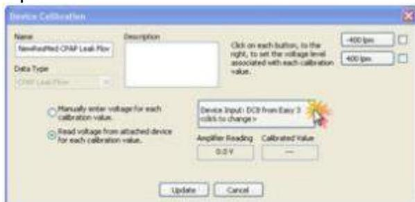
9. To Calibrate the Low Value - Set the DC device (in this example the DC device is a ResMed flow channel) to the lowest flow/calibration setting. Click on the -400 lpm button. Proceed forward until the following prompt is displayed. If you would like to
