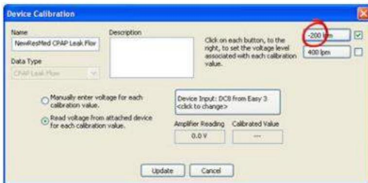
11. To Calibrate the High Value - Set the DC device (in this example the DC device is a ResMed flow channel) to the highest flow/calibration setting. Click on the 400 lpm button. Proceed forward until the following prompt is displayed. If you would like to specify a different low calibration value (the default was 400) you can enter it in the calibration value field. In the example below, the calibrated value (400) will be manually modified to 200. Click on Update to continue.
