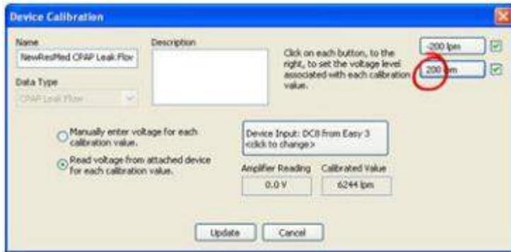
13. The new DC calibration should now be displayed in your list of DC input calibrations. (Note the illustration below)
