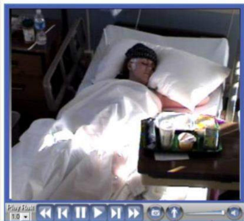
Q-Video is a digital video recorder and player designed by the Cadwell development team in Kennewick, Washington. The software has a motion detection algorithm that detects movement from a video signal. Movement can be accentuated with color and displayed in the video picture to assist clinicians in detecting subtle movements. All video is time synchronized with recorded waveform data.
