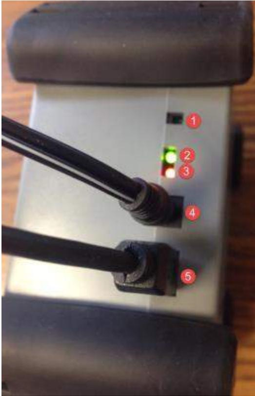
1. Power on/off button. Insert tool provided into the slot and press and hold until unit turns on.
