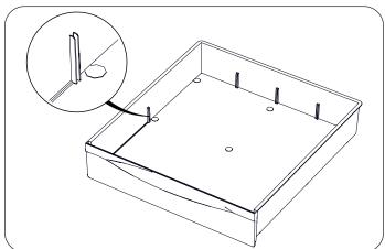
2. Install the short divider with 3 notches facing upward.
