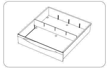
3. Note the divider ribs located on the front and rear faces of the drawer.
