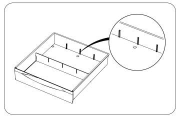
4. Install the 3 long dividers with notch facing downward.
