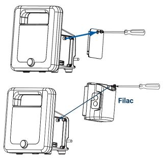
Optional modules ordered at the time of original purchase are installed prior to shipping. Modules can also be ordered later and installed in the field. To install the Covidien Filac™ temperature module, use the included Phillips head screwdriver to remove the panel cover on the right side of the unit (the right side when the screen is facing the user). Attach the module and fasten in place. Insert the probe/well assembly into the top of the module.
