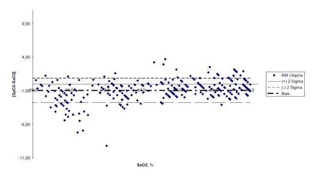
The tested device meets the stated accuracy specification of RMS Error = 1.89% for the range 70% to 100% SaO<sub>2</sub>. The accuracy is not specifed below 70% SaO<sub>2</sub>. In addition, here are detailed measured A<sub>RMS</sub> values over the specified discreet ranges:
