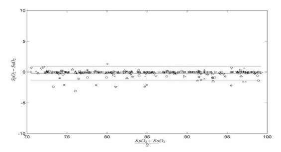
The tested device meets the stated accuracy specification of RMS Error = 2.00% for the range 70% to 100% SaO<sub>2</sub>. The accuracy is not specified below 70% SaO<sub>2</sub>. In addition, here are detailed measured A<sub>RMS</sub> values over the specified discreet ranges:
