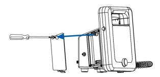
Optional modules ordered at the time of original purchase are installed prior to shipping. Modules can also be ordered later and installed in the field. To install an SpO2 module, use the included Phillips head screwdriver to remove the cover on the left side of the unit (the left side when the screen is facing the user). Attach the module and fasten in place.
