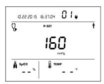
Example shows Manual Mode setup display. Three-digit number is the target cuff inflation pressure setting. The default is 160 mmHq.
