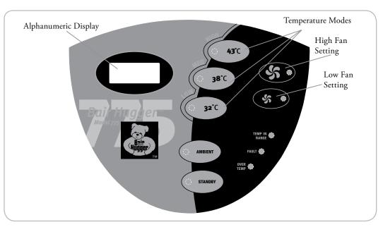
Figure C. Model 775 temperature management unit control panel
