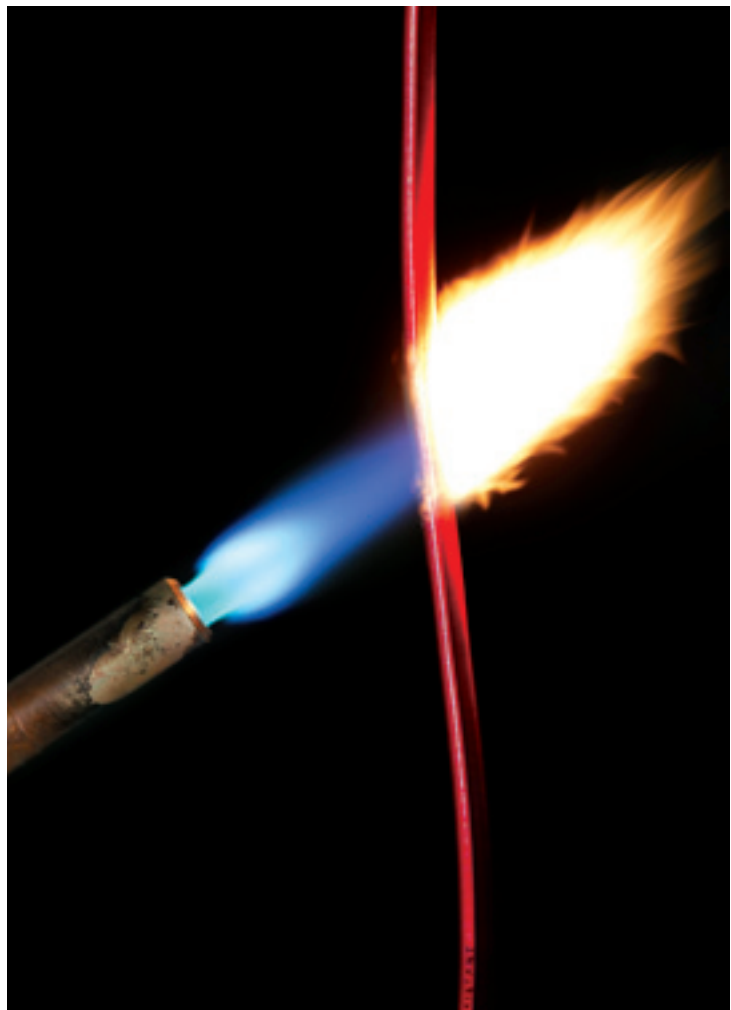
(* VW-1: Vertical Single Wire Flame Test)
