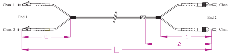
Fig. 2: Duplex patchcord schematic
