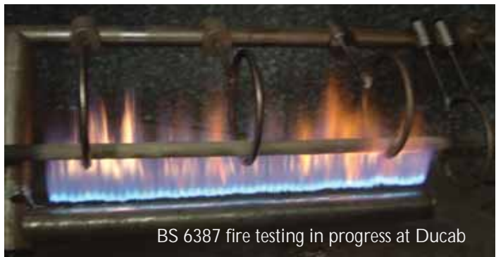
Fire Test after 6 minutes
