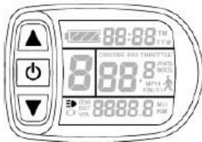
Hold long to turn on headlights (the controller should have headlight drive output function); hold long again to turn off the headlights.
