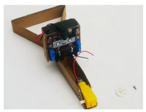
Screw in the circuit board onto the front of the box using the four smaller bolts, with nuts, with the nuts on the front. Then get the battery box fitting snugly inside!
