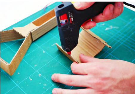
Now we need to make the box that will hold our Smartibot circuit board and its batteries. Glue along both of the edges and stick the two pieces together.
