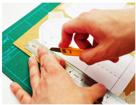
Now, using a ruler and a craft knife, it's time to cut out those cardboard shapes along the solid lines shown on the templates.
