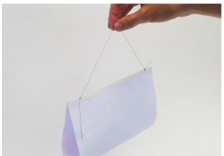
With the cradle made, we just need to attach it to the crane using the pulley. Cut a 125 cm long piece of thread and tie a knot around the thread that is attached to the cradle, to connect them.
