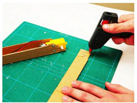
Now apply a zig zag pattern of hot glue on the tabs at the ends of the assembly you have just made. Glue it to the neck, then do the same for the other side. Remember to hold the pieces together for several seconds so the glue has a chance to cool and solidify!
