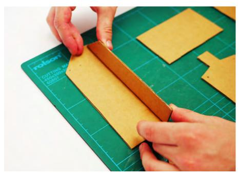
With all the cardboard shapes cut out, it's time to fold! Fold along the lines you pushed in with the ruer earlier. Don't worry about them staying folded, glue or screws will hold things together later.
