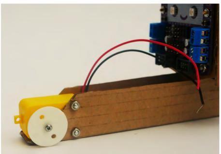
Use a small screw and a screwdriver to attach the wheel mount to one side of the motor. You choose! We will use the wheel mount as the crane's pulley.
