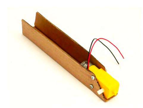
Taking the neck, the long bolts, nuts and the motor and attach the motor to the neck as shown:
