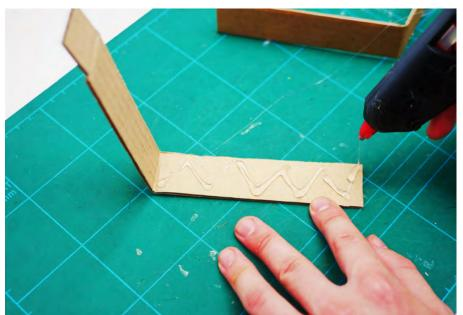
Putting the neck with the motor to one side for now, it's time to get gluing. Use the glue gun to glue a zig zag pattern onto one of the long rectangular pieces, and then stick it to the other one. Hold them together for a few seconds to get a strong bond!
