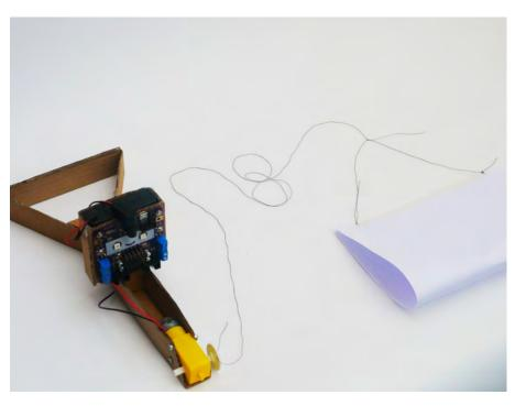
Then thread the other end of the longer piece of thread through one of the holes in the wheel mount, as shown.
