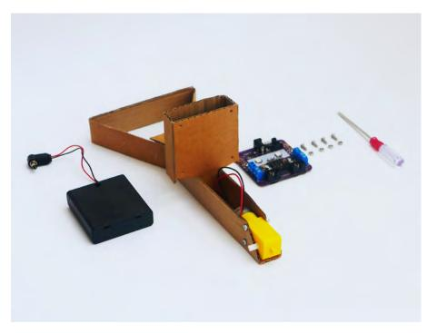
Now you've made the cardboard chassis for your crane it's time to make it work by adding the Smartibot circuit board and battery box.
