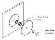
To install the glass piece, hold the glass against the LED housing and thread the 30mm threaded cap into the LED housing.
