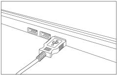
Insert the larger end of the Micro USB charging cable into a USB wall charger for a Smartphone or iPhone (5V  $\rightleftharpoons$  1.0A up to 5V  $\rightleftharpoons$  2.4A maximum), or a USB port on your laptop/computer to charge the OontZ Angle 3 battery.
