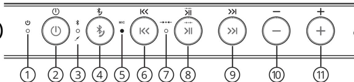
1. **Charging Indicator Light (Red)** - Flashes red when charging, solid red when fully charged
