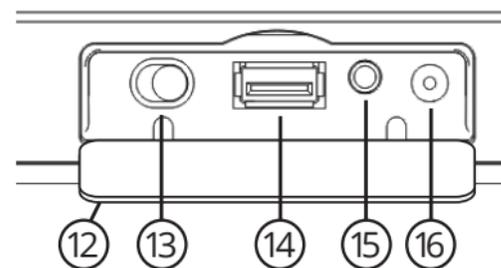
12. **Connector Flap which can be lowered down** - Inputs are located on the rear of the speaker underneath this flap
