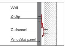
Note: Ensure the the z-clips are fixed in the same direction on all the panels.
