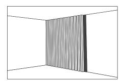
Note: Ensure the screws are of the right size and can hold the panel in place. Fire the screws into the second panel only after the lip and recess are fit properly. Fire the screws through the acoustic polyester baseboard and not through the wooden slat.
