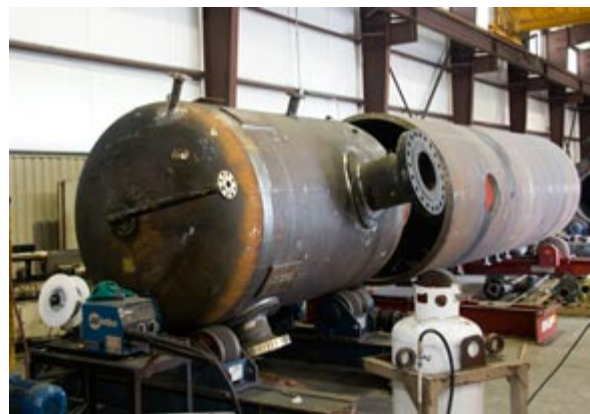
A pressure vessel in the mid-fabrication stages.
