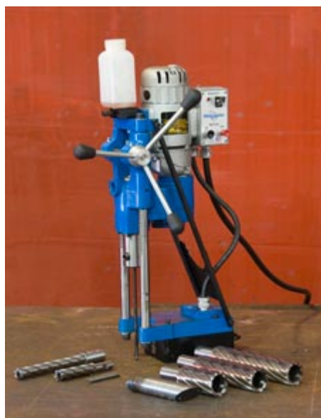
Hougen HMD915 magnetic drill and the Rotabroach® Industrial Cutters that are used for both the 1" and 2" diameter holes.
