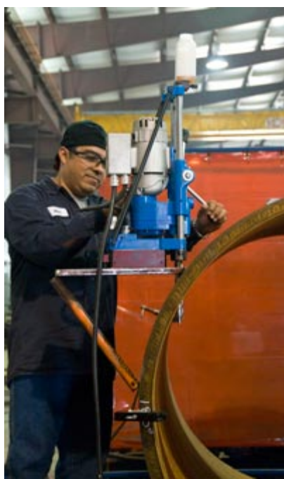
Hougen HMD915 magnetic drill cutting a hole on 2" thick pressure vessel.
