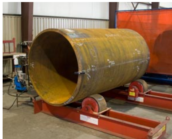
Shell of new pressure vessel at the early stage of fabrication.
