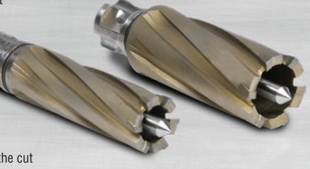
Slot allows coolant to flow to the cutting teeth
