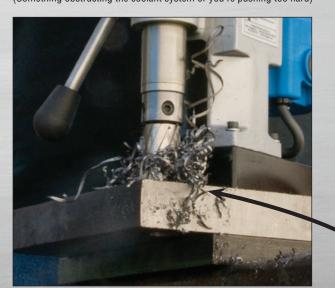
The cause of cutters quickly cutters quickly dulling is too little dulling is too little feed pressure.
